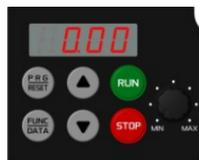
Figure 4.2 Display of the LED Monitor
